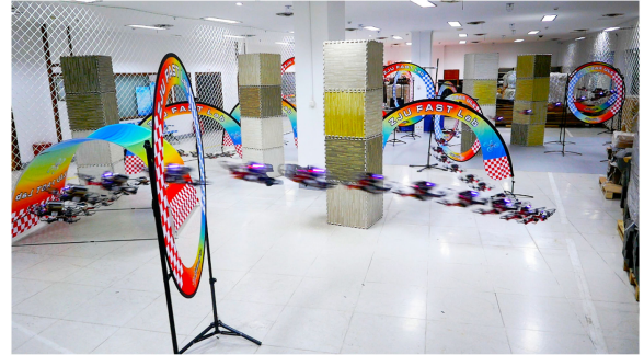
Fig. 1. Composite image of the quadrotor aggressive flight in a limited space. Our quadrotor is equipped with a stereo camera, an IMU and an onboard computer. No external positioning system is used. A video of the experiment can be viewed at https://youtu.be/H89ALyWA2NI .
